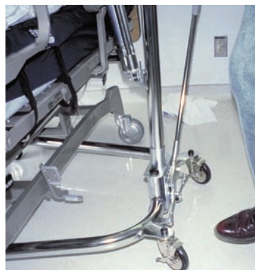
FIGURE 36-41 Spread the base of the hydraulic lift to provide stability. DELMAR/CENGAGE LEARNING
