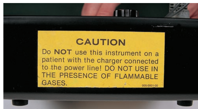
FIGURE 29-8 Warning Label on Electrical Equipment DELMAR/ CENGAGE LEARNING
