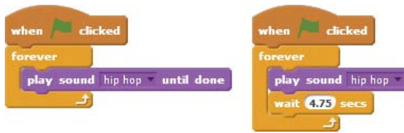
Figure 3-7: Two ways to create background music: Repeat the sound after it finishes (left) or start the sound over after playing it for a certain amount of time (right).
