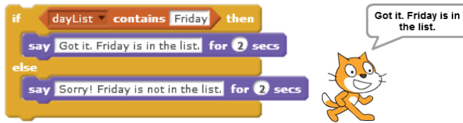
Figure 9-9: Using the contains block to check whether a string is in a list
