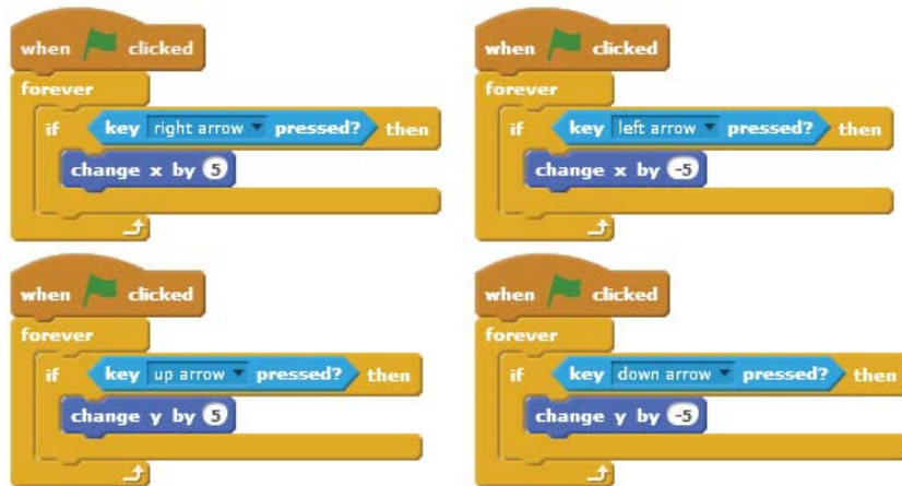
Figure 7-5: These scripts allow you to move a sprite using the keyboard arrow keys. Each script responds to one of the four keys.
