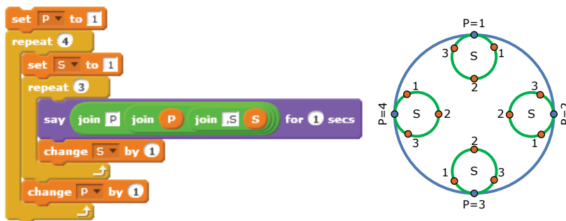
Figure 7-15: Visualizing nested loops. The variable P controls the outer loop and the variable S controls the inner loop.
