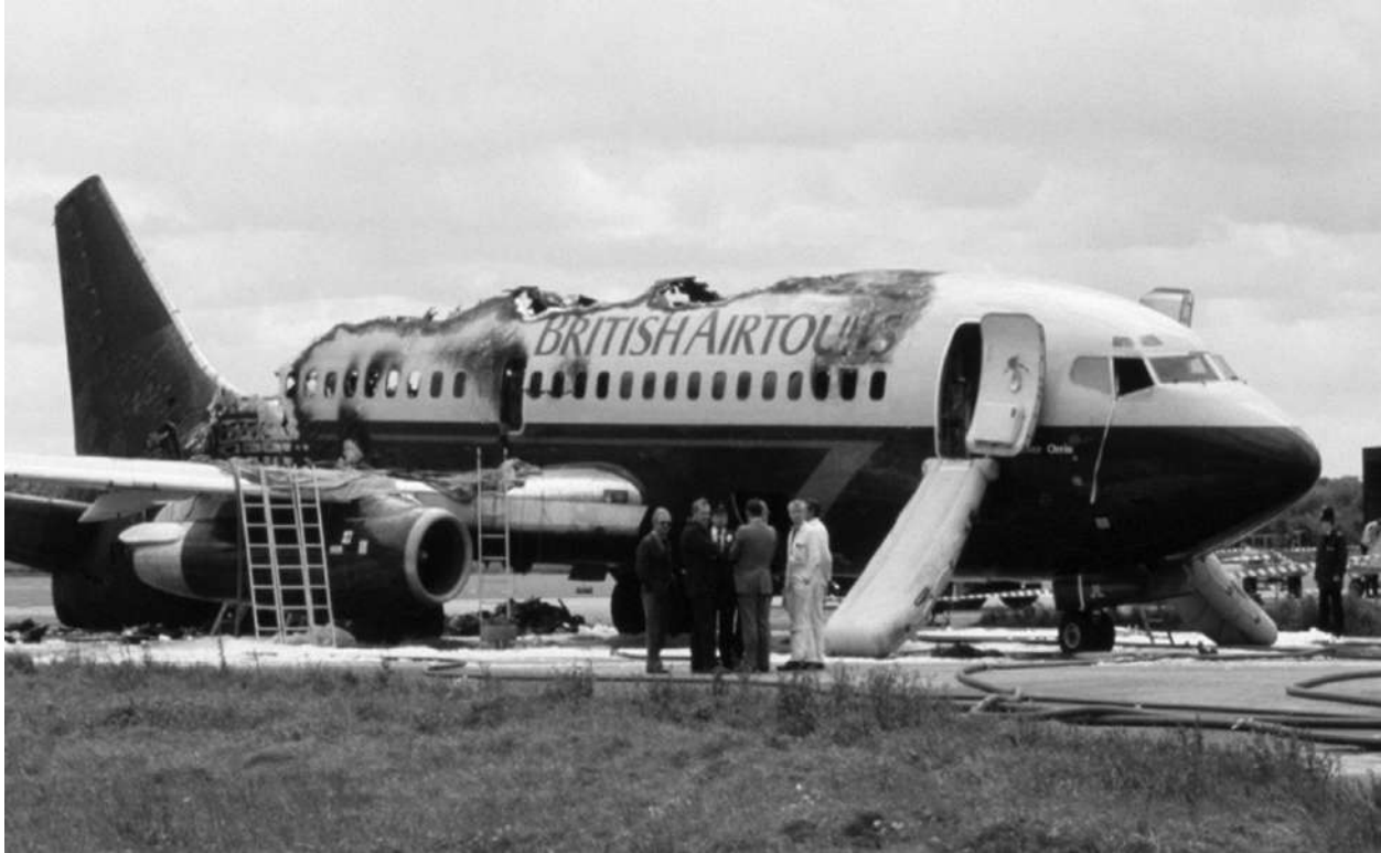
FIGURE 2-9 Wreckage showing evidence of fire and a ground evacuation. (Source: U.K. Air Accidents Investigation Branch)
