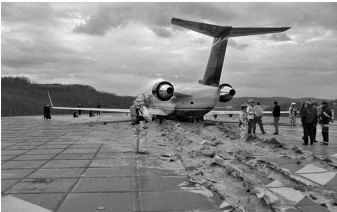
FIGURE 9-7 Concrete blocks from the EMAS crushed under the weight of the PSA Airlines plane. (Source: NTSB)
