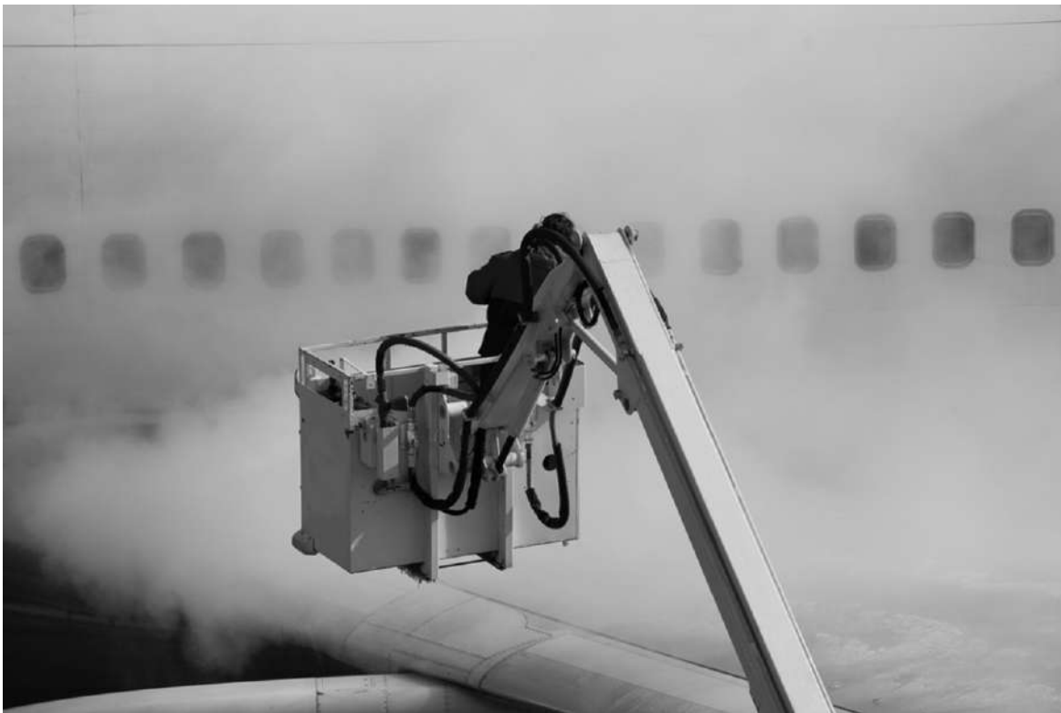
FIGURE 9-4 Personnel deicing the wings of an aircraft prior to takeoff. This is essential since wing icing can adversely affect the aerodynamics of a plane. (Source: Wikimedia Commons )
