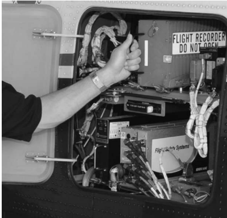
FIGURE 7-2 A crash survivable FDR can also be used for FOQA. (Source: Authors)
