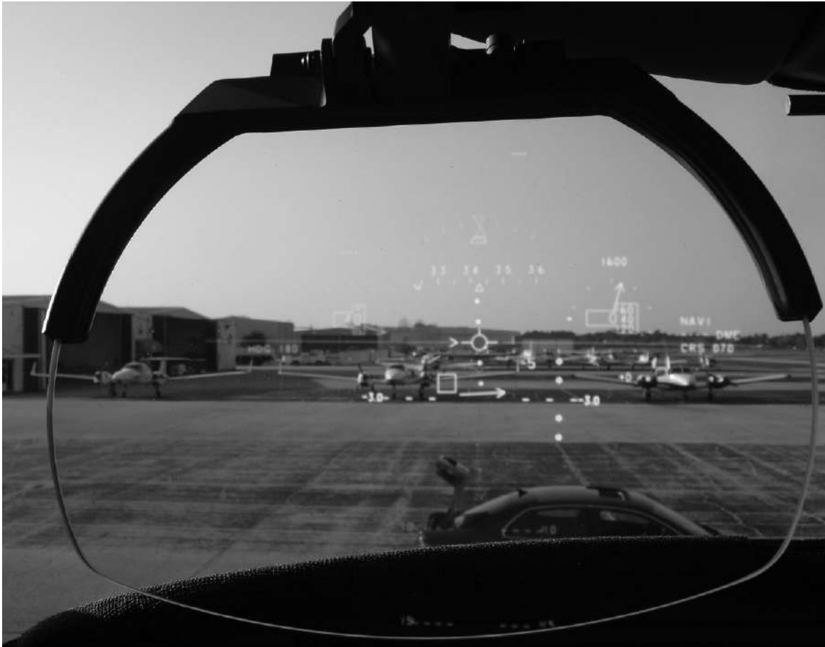
FIGURE 8-6 The view through a HUD while parked on a ramp. (Source: Authors)
