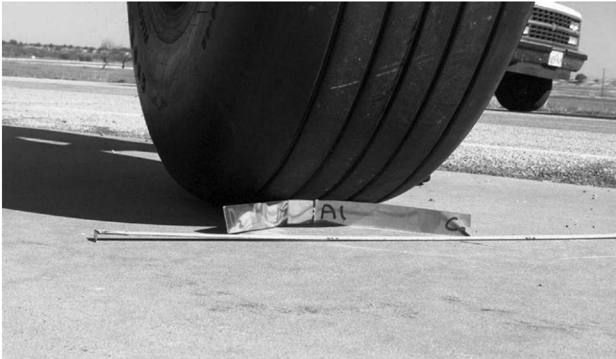
FIGURE 2-20 Analyzing the impact of the metal strip to the Air France Flight 4590 tire. (Source: French Bureau Enquêtes-Accidents )
