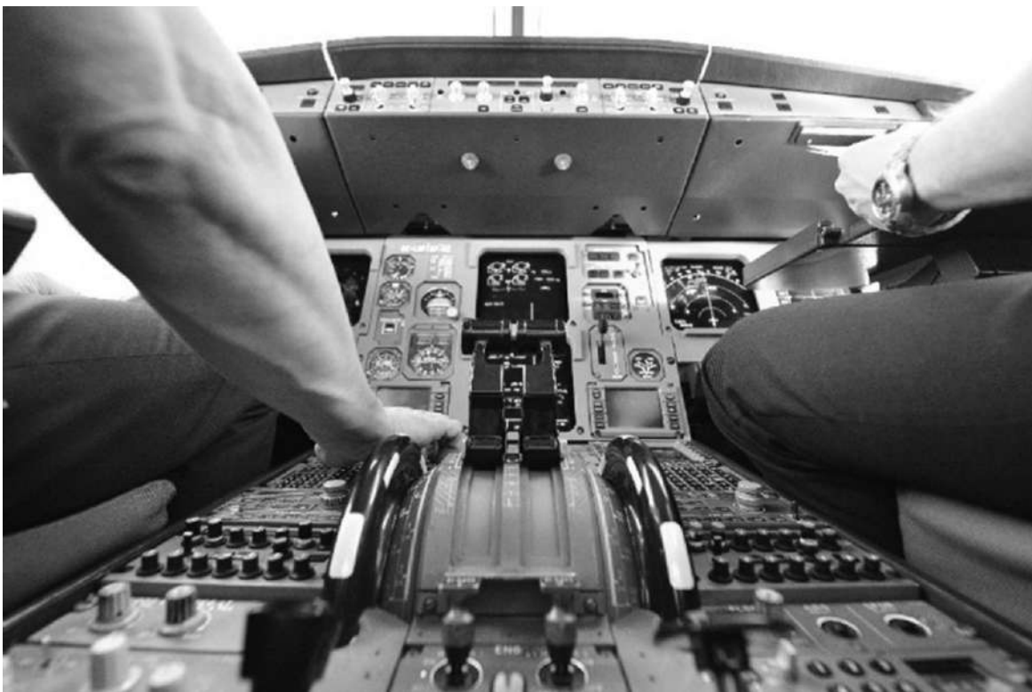
FIGURE 7-1 Instrument readings and control inputs are routinely captured for FOQA analyses. (Source: Wikimedia Commons )
