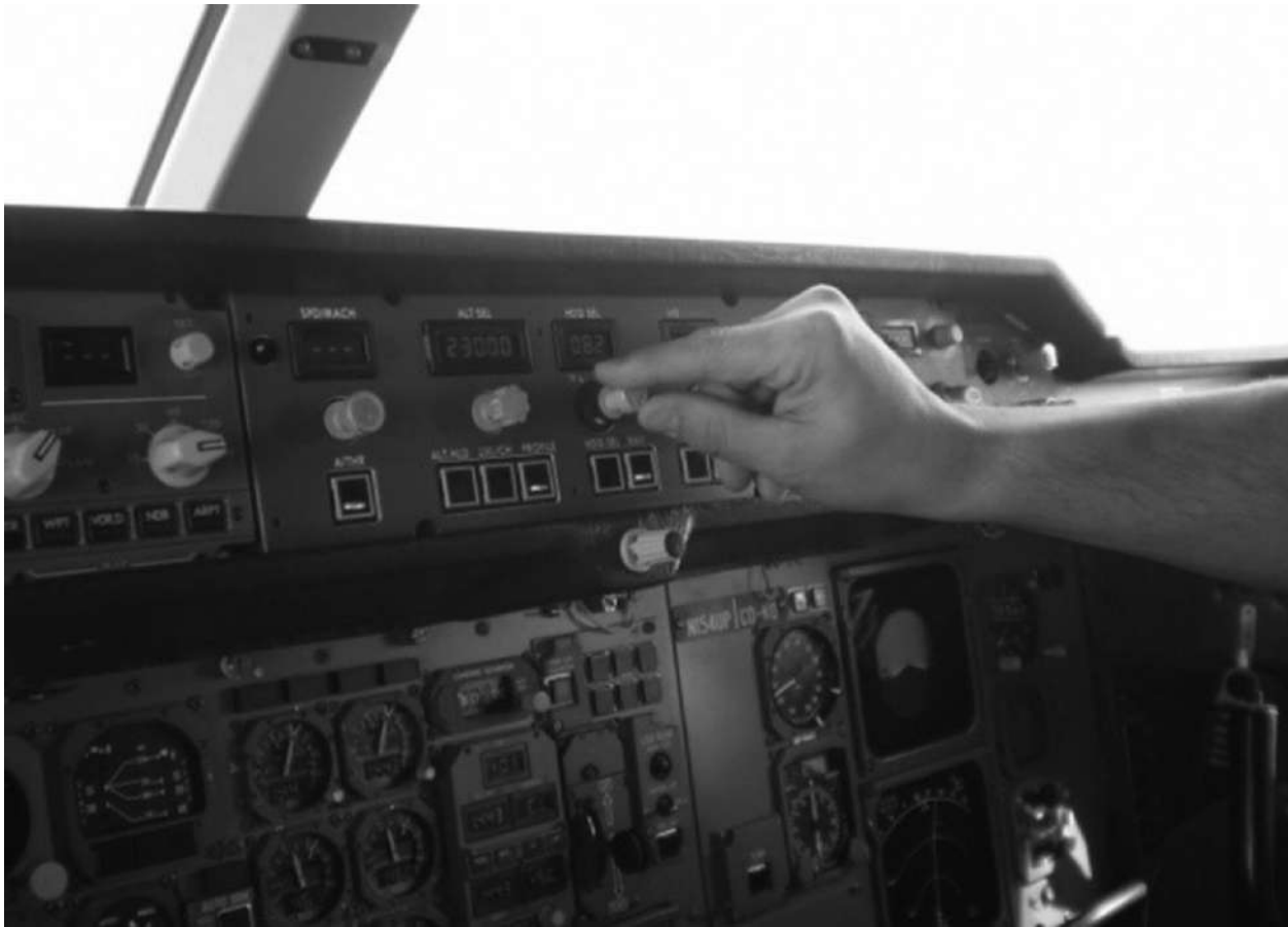
FIGURE 8-3 Pilots are taught to look for an output to an input, meaning that the pictured pilot may be moving a heading knob but looking at a flight display instead of the knob to see the actual output of the change. (Source: Authors)
