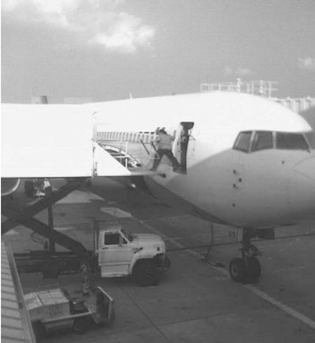
FIGURE 1-6 An aircraft catering agent is seen leaping over a large gap between the plane and the ramp. This is not a practice of good safety! (Source: Authors)
