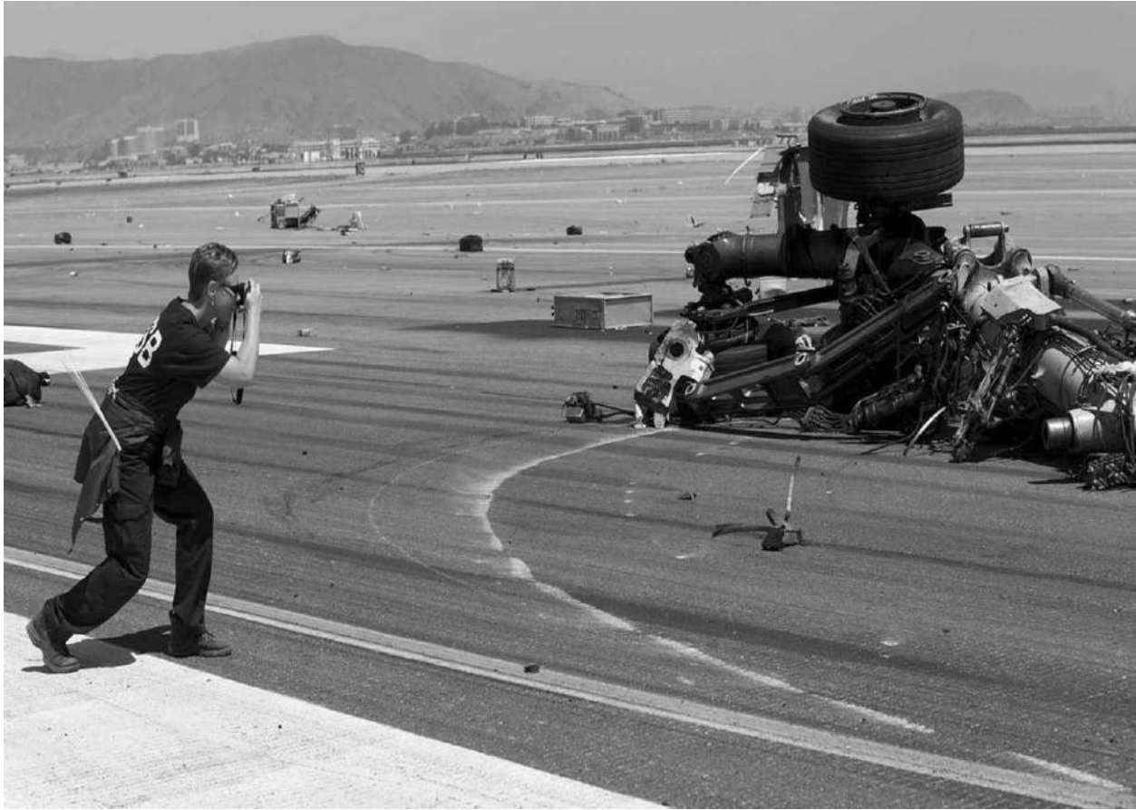
FIGURE 1-5 An investigator from the NTSB taking pictures of a landing gear from Asiana Flight 214 in San Francisco. (Source: NTSB)
