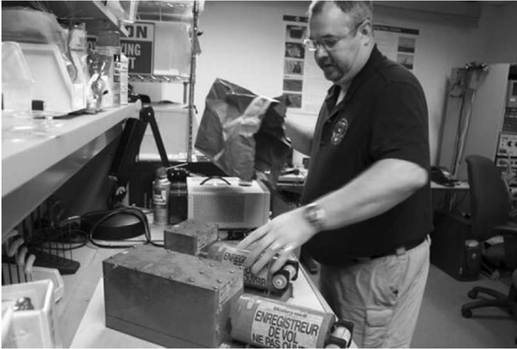
FIGURE 6-6 Receiving the CVR and FDR (black boxes) from Asiana Flight 214 for analysis. (Source: NTSB)
