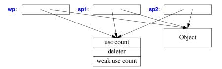
The "weak use count" is needed to keep the use count structure alive because there may be weak ptrs after the last shared ptr for an object (and the object) is destroyed.
