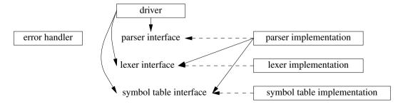
A dashed line means "implements." I consider this to be the real structure of the program, and our job as programmers is to represent this faithfully in code. That done, the code will be simple, efficient, comprehensible, maintainable, etc., because it will directly reflect our fundamental design.
