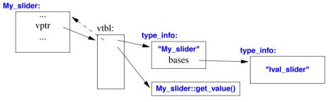
The dashed arrow represents an offset that allows the start of the complete object to be found given only a pointer to a polymorphic subobject. It is clear that **dynamic\_cast** can be efficiently implemented. All that is involved are a few comparisons of **type\_info** objects representing base classes; no expensive lookups or string comparisons are needed.
