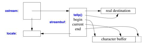
The set of template arguments for an **ostream** and its **streambuf** must be the same, and they determine the type of character used in the character buffer.
