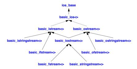
The classes suffixed by  $\diamond$  are templates parameterized on the character type. A dotted line indicates a virtual base class (§21.3.5).
