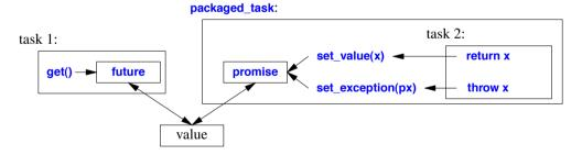
We pass a task (a function or a function object) that we want executed to a packaged\_task. When our task executes a return x, it causes a set\_value(x) on the packaged\_task's promise. Similarly, a throw x causes a set\_exception(px) where px is an exception\_ptr for x. Basically, the packaged\_task executes its task, f(args), like this:
