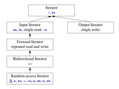
The iterator categories are concepts (§24.3) rather than classes, so this hierarchy is not a class hierarchy implemented using derivation. If you need to do something advanced with iterator categories, use iterator\_traits (directly or indirectly).
