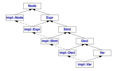
That worked but led to excessive memory overhead: the nodes were too large because of data needed to navigate the virtual bases. In addition, programs were seriously slowed down by the many indirections to access the many virtual bases in each object (§21.3.5).
