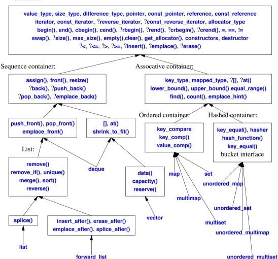
An arrow indicates that a set of operations is provided for a container; it is not an inheritance operation. A question mark (?) indicates a simplification: I have included operations that are provided for only some of the containers. In particular:
