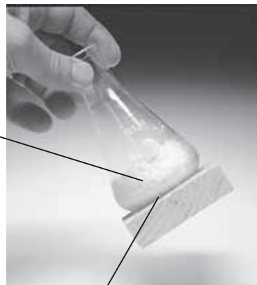
The chemical reaction happening in the flask is endothermic. It absorbs energy from the flask, the wood, and the air.
