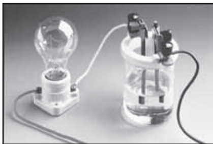
Pure water does not conduct an electric current.
