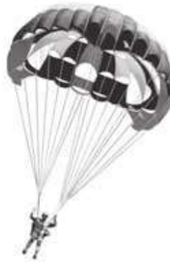
The parachute increases the air resistance of this sky diver and slows him to a safe terminal velocity.
