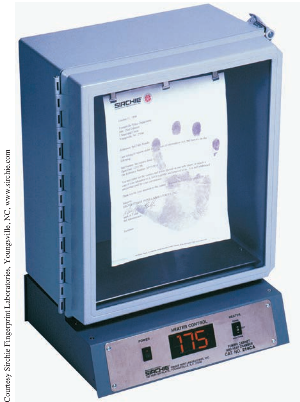
FIGURE 6-14 A heated fuming cabinet.
