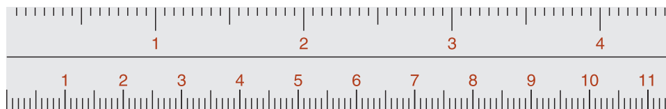
Comparison of the metric and English systems of length measurement; 2.54 centimeters = 1 inch.
