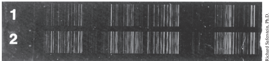
A comparison of paint chips 1 and 2 by emission spectrographic analysis. A line-for-line comparison shows that the paints have the same elemental composition.
