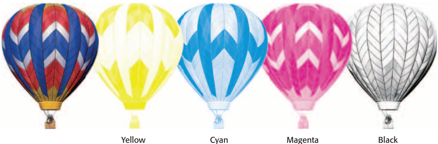
Figure 10 The picture of the balloon on the left was made by overlapping yellow ink, cyan ink, magenta ink, and black ink.
