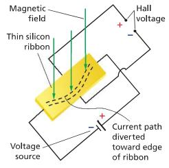
A magnetic field forces more electrons to the edge of a thin metal strip. This creates the Hall voltage.
