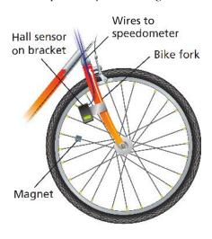
Bicycle speedometers use a Hall-effect sensor to display the speed at which a bicycle is moving.
