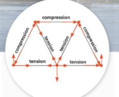
A bridge works by balancing compression (pressing inward) and tension (pressing outward), distributing the load onto the bridge supports.
