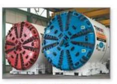
Engineers used tunnel boring machines like the ones shown above to dig an extension of the Metro Gold Line in Los Angeles. The tunnels are 1.7 miles long and 21 feet wide.
